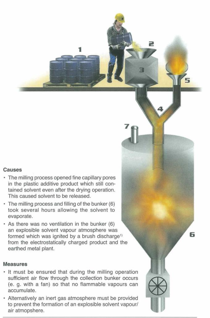
Brush discharges are not incendive for dust/air atmospheres provided no flammable gases or vapours are present.
