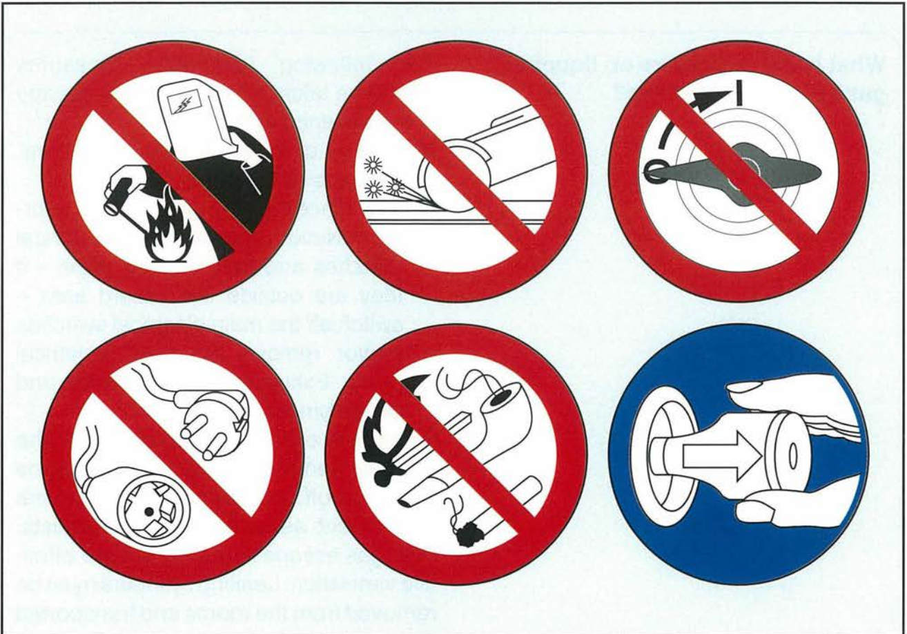
Fig. 45: Avoidance of ignition sources on gas escape
