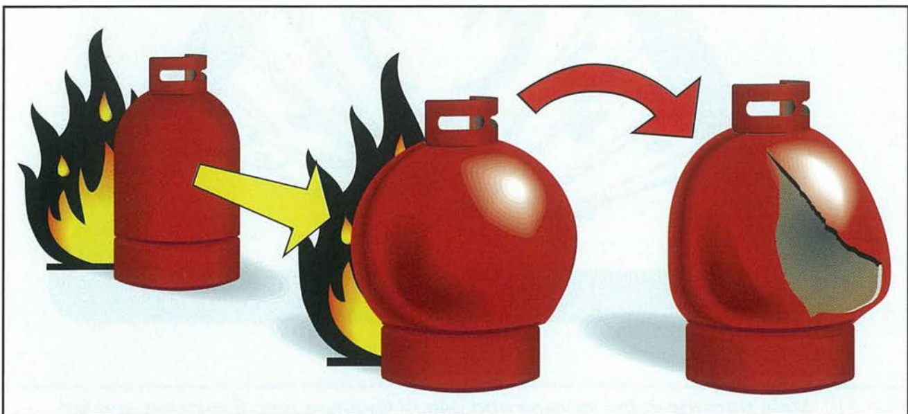
Fig. 12: Effect of fire on a liquefied gas cylinder
