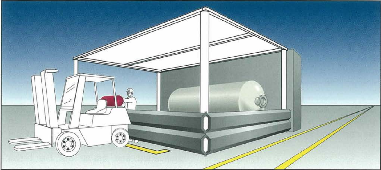
Fig. 29: Protection of the supply facility against mechanical damage
