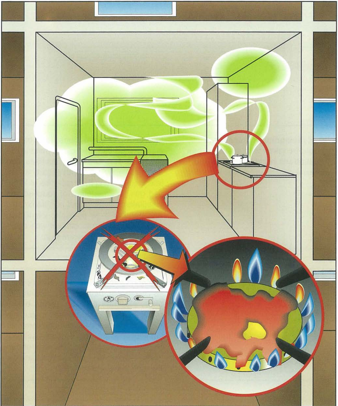
Fig. 17: Formation of carbon monoxide due to a dirty stove
