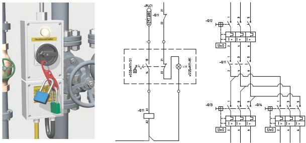
Figure 2: Maintenance switch, operating indirectly with signal lamp
