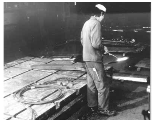
Fig. 2: Hoses are properly coiled up next to the working area thus eliminating a trip hazard.
