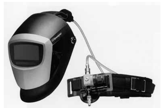
Fig. 4: If thermal cutting or flame heating processes are to be carried out in confined or poorly ventilated areas (e.g. in containers, pipes), a compressed air line breathing unit together with a welding helmet must be worn.
