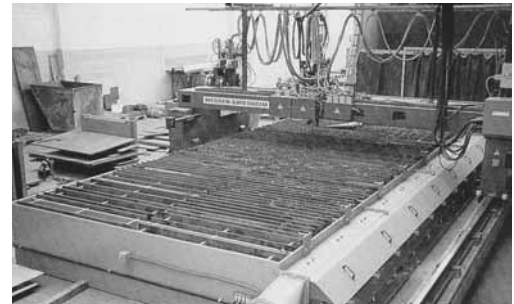
Fig. 3: Gas cutting workplace with extraction system at the worktable (multi-chamber extraction system) and dust removal system.
