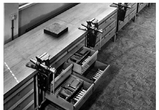
10 Ideally, each worker is provided with his personal set of hand tools and a dedicated place where they are kept.
