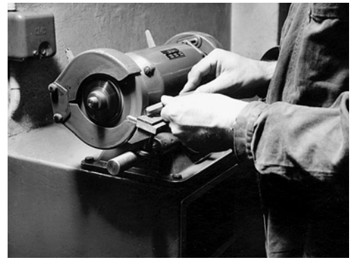
6 Ensure that any mushroomed heads are ground off immediately. The head's striking face must be slightly rounded or chamfered.
