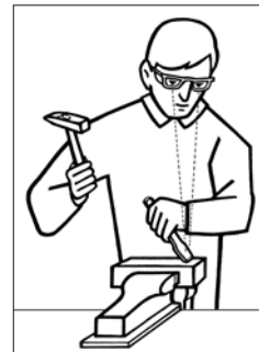
9 Correct chiselling technique: workpiece clamped in bench vice, hammer held correctly, cutting edge visible, safety goggles are being worn.
