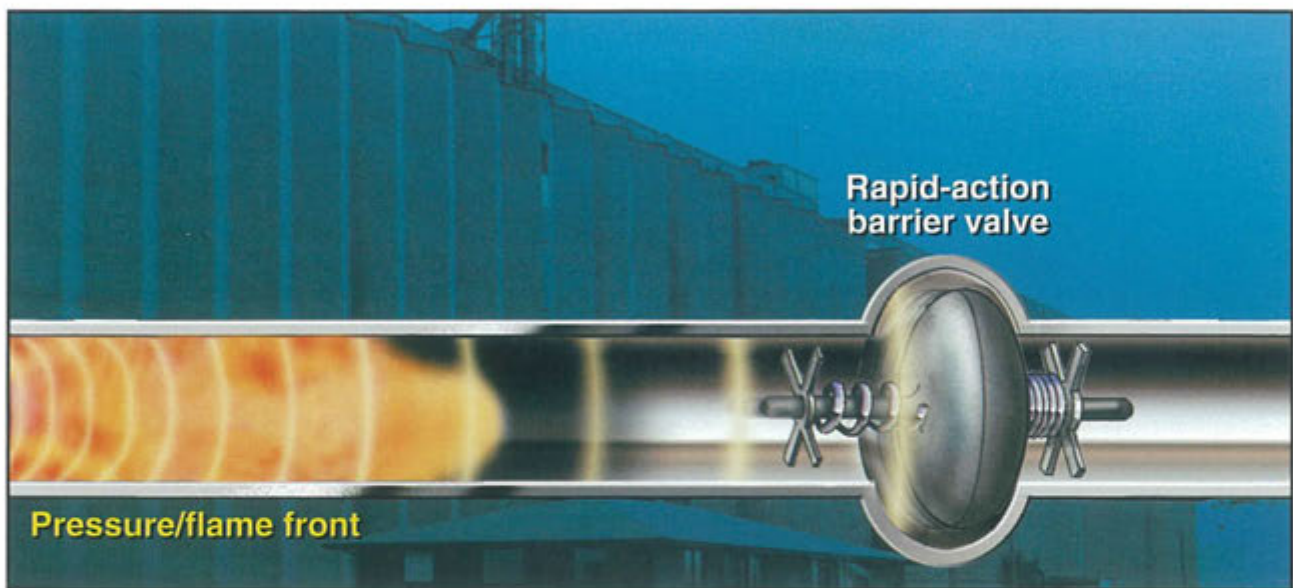
Fig. 22: Rapid-action barrier valve (passive device)
